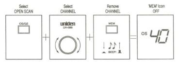
The selected channel has now been removed from the scan group and will not be included when scanning has commenced and the **MEM** indicator will not be displayed on that channel.
